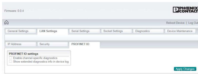
Figure 3-6 “LAN Settings/PROFINET IO” page
